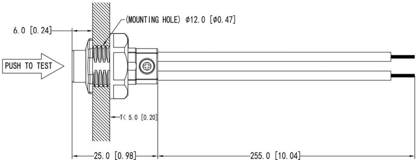
Dimension in millimetres [inches in brackets]
