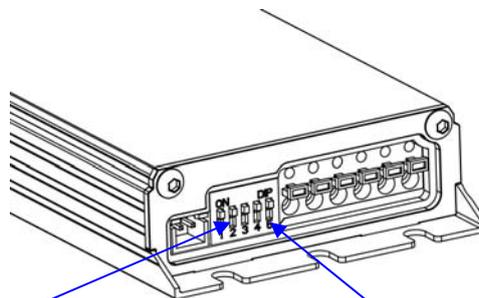
Dipswitch 1/2/3: Setting LED working current in normal mode
